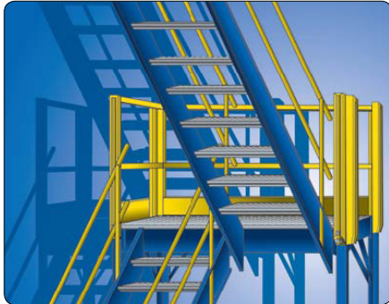
The 180-degree turn plat-form is used in tight areas to conserve space.
