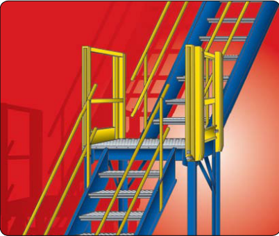
Platform landing is used for straight through passage with stairway proceeding upward.
