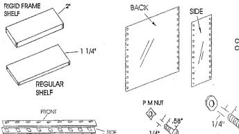
1/4 X .58 SHOULDER BOLTS AND P M NUTS USED FOR INSTALLING RIGID FRAME SHELVES.
