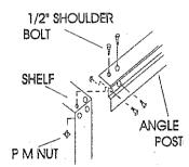
Insert shoulder bolt thru post hole and shelf hole (Fig.1). Connect 4 point lock nut (Fig.2) and tighten shoulder bolt (Fig.3). When all connections are completely tightened, this unit forms a rigid structure.
