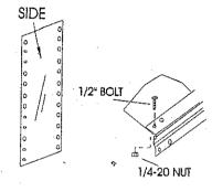
Sides made in two pieces should overlap 3" in the center and be flush with the post ends on top and bottom.
