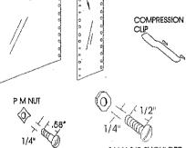
BOLTS AND HEX NUTS USED FOR INSTALLING BACKS, AND SIDES
