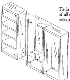
Tie in top and bottom of all units with 1" bolts and nuts.
