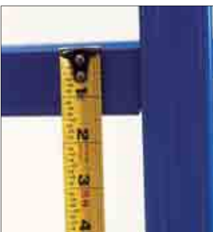
Low profile shelf beams are 1/2" high and adjustable on 1/2" centers.
